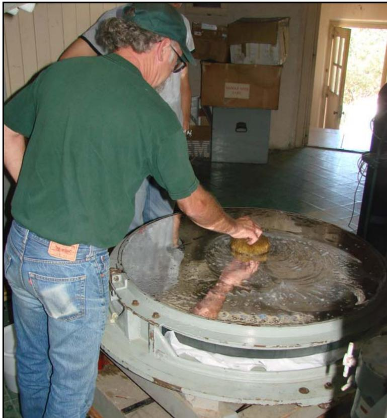
We washed the mirror in the cell using as little water as we could. The band for removing the mirror from the cell is missing so washing in the cell is necessary. Just be prepared for the water cleanup under and around the cell.
