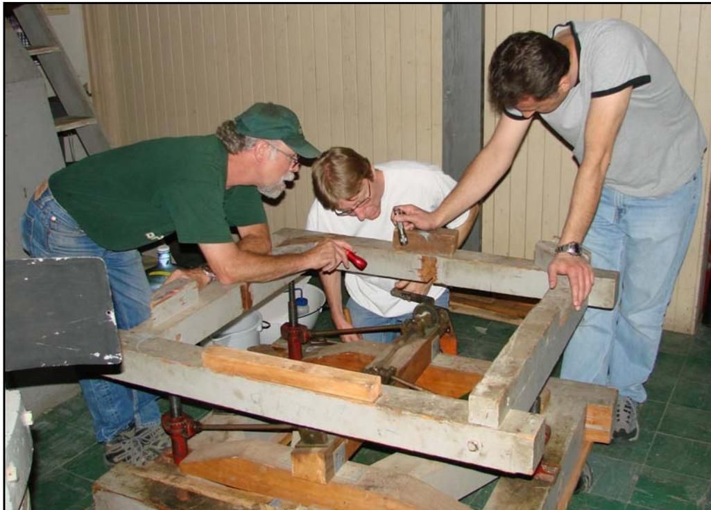
We had a broken tapered pin in the crank assembly of the mirror removal fixture. It pays to test before it is positioned under the mirror.
