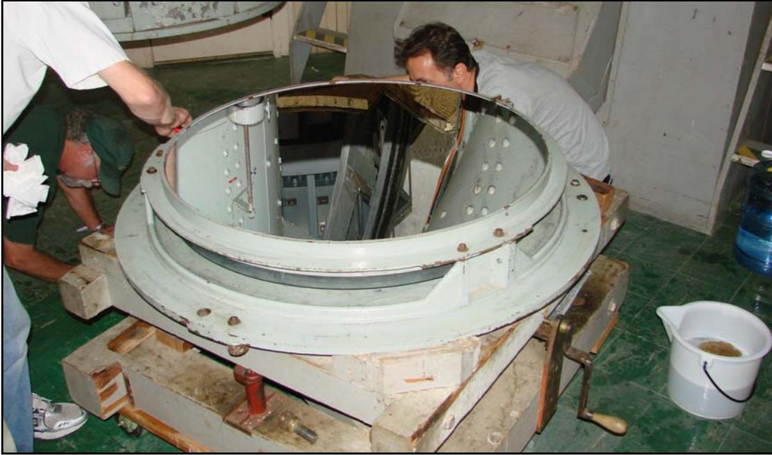
Drying the cell and floor after drying the mirror with blotter paper.
