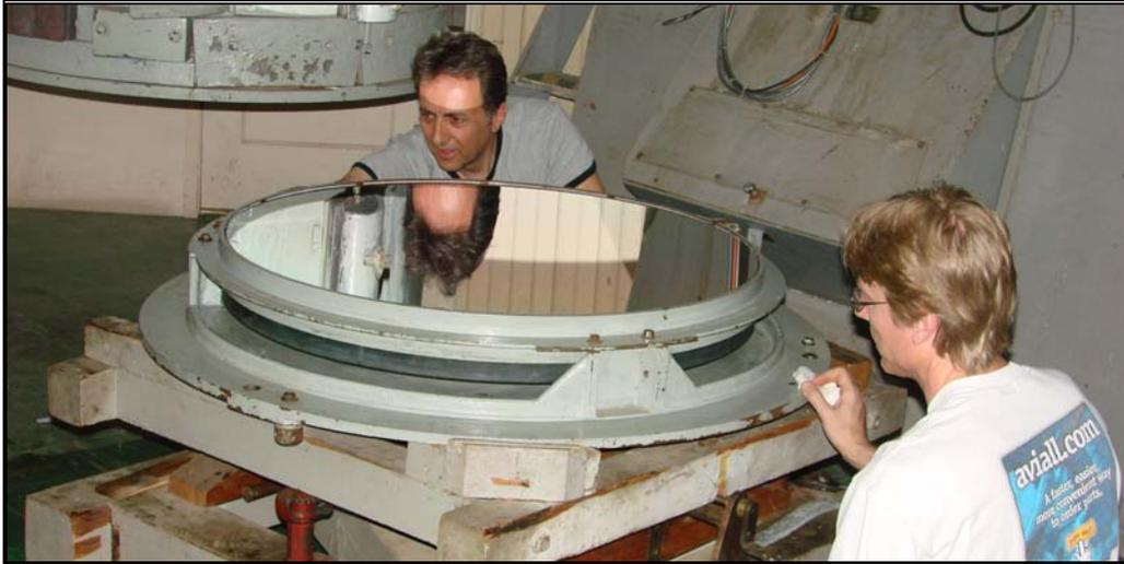
To start, install the RA support post. The top of the post has a rounded cutout that cradles the small weights on the end of the shaft. Use the wedge blocks to adjust the support height to level out the mirror cell and support the weight of the telescope once the mirror cell is removed.
