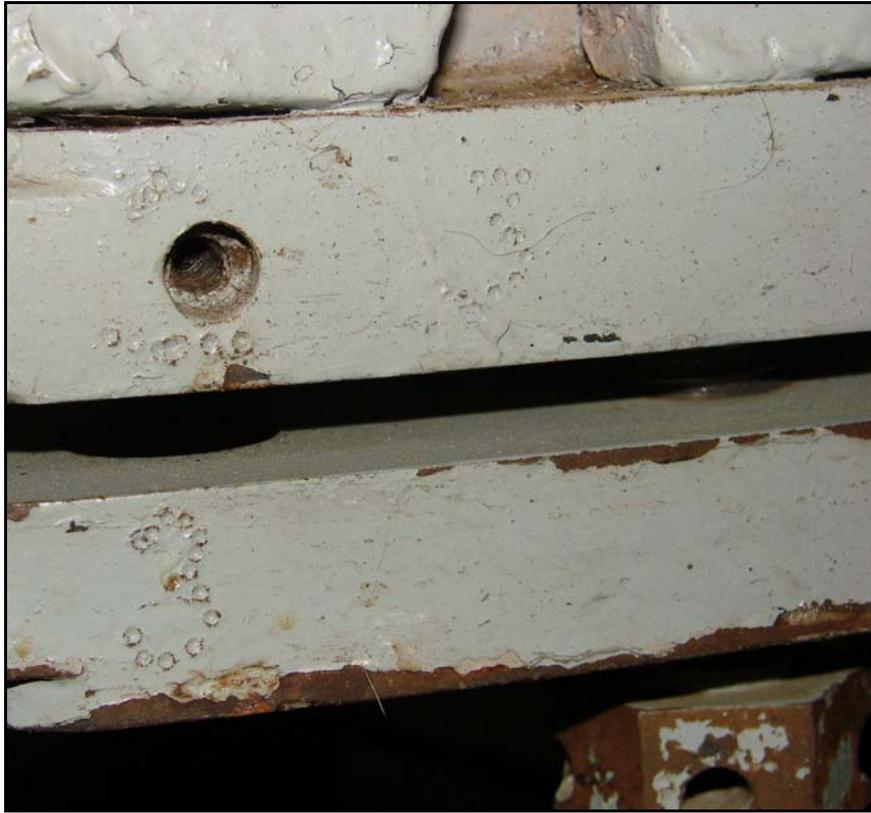
The mirror cell and mounting flange on the telescope are numbered for alignment purposes. This image shows position number three. There are a total of three mounting bolts to attach the cell.
