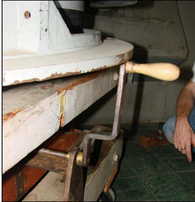
Make sure the mirror fixture is positioned so the crank clears the cell while lowering. We had to remount the cell and reposition the fixture.
