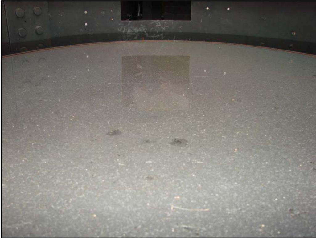
The telescope has not been used for a couple of years and even though covered has gotten quite dirty. This is an image of the dirty pre-washed mirror taken at a low angle through an access port. The mirror is SiO overcoated.
