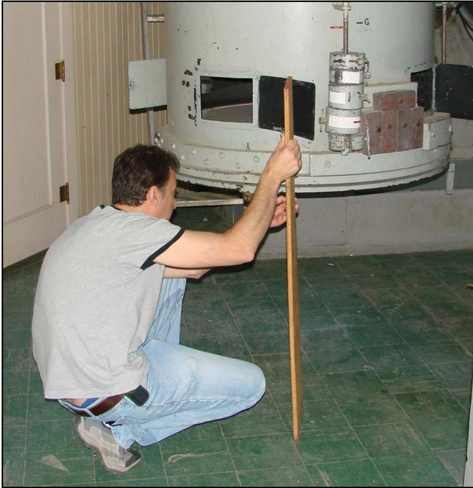
Level the mirror cell and lock the DEC motion.
